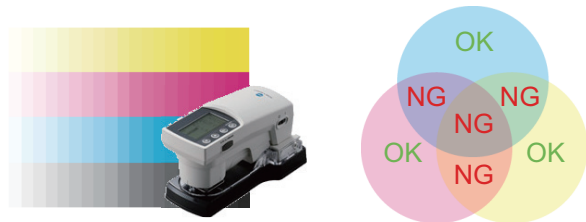
Fig. 11 Conventional calibration calibrates primary color gradations only, and is unable to calibrate color balance deviations.
